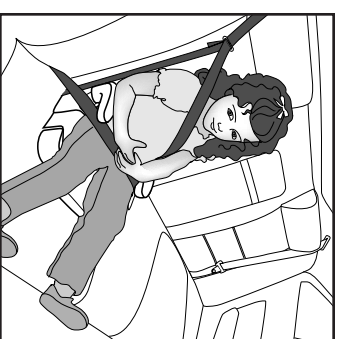
14. Backless booster seat: belt positioning strap with child
