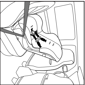
6. Rear facing convertible seat: installed
